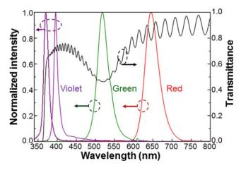
Yao, Yang and Teng et. al. <sup>24</sup>, specified the effective illumination spectral range for causing AgNP aggregation using light-emitting diodes (LEDs) of designated wavelengths. Their adjacent figure shows the transmission spectrum of a fresh AgNP sample. They reported the greatest transmission of AgNPs light energy occurred "around 520 nm in wavelength," corresponding to the LSPR. "The emitted spectral peaks of
